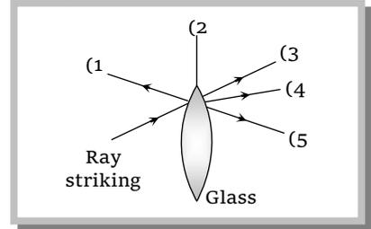
205 From shows five rays from an object passing through a converging lens. There of these rays are correctly drawn. The two rays, not drawn correctly, are
