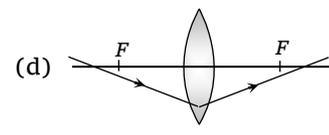
204 A ray of light strikes a piece of glass shaped as shown in figure. Along which path does the ray continue
